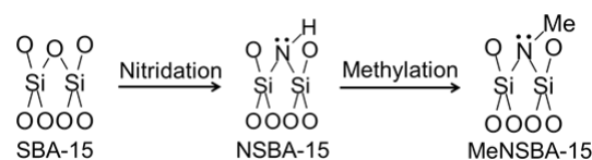
Fig. 1 Formation of nitrogen-substituted and N-methylated silica (SBA-15)
