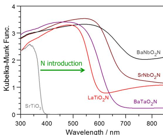
**Figure 1.** UV-vis DRS spectra of perovskite oxynitride photocatalysts,  $ABO_2N$  (A=La, Sr and Ba and B=Ti, Ta and Nb).
