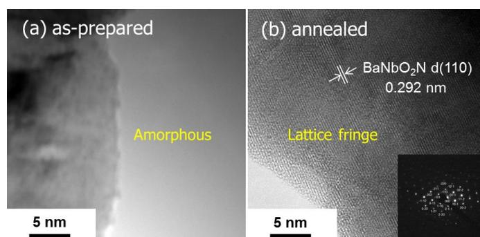
**Figure 2.** HRTEM images of  $\text{BaNbO}_2\text{N}$  particles (a) as-prepared by the nitridation at 1173 K for 20 h and (b) subsequently annealed in a Ar flow. SAED patterns in (b) indicate diffraction of  $\text{BaNbO}_2\text{N}$  along the [110] zone axis. (a) was reprinted from ref. 4.
