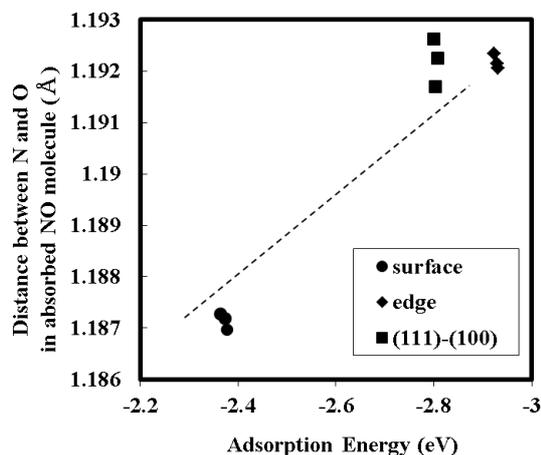
Figure 2. Relationship between bond distance and adsorption energy of NO on  $\text{Rh}_{55}$  nanoparticle.
