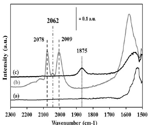
Figure 1. FT-IR spectra of adsorbed species on Rh single-nano catalyst. (a) 700 ppm NO/He for 5 min. after oxidation treatment, (b) 1 % CO/He for 5 min. after 700 ppm NO/He, (c) 700 ppm NO/He for 5min. after 1 % CO/He flow.
