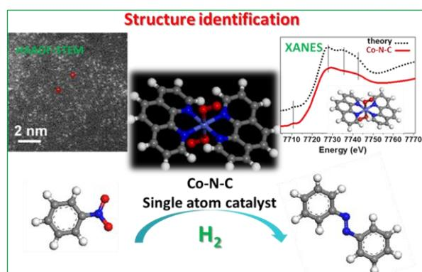
**Figure 1.** Atomically dispersed Co-N-C catalyst.
