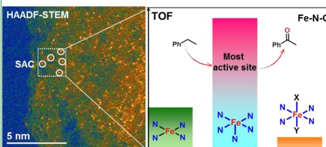
**Figure 2.** Atomically dispersed Fe-N-C catalyst
