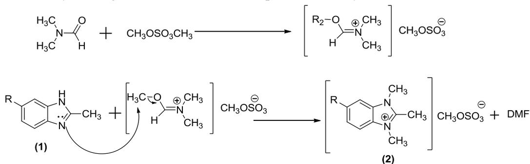
**Figure 1.** Synthesis of methoxymethylene-N,N-dimethyliminium methosulphate salts.
