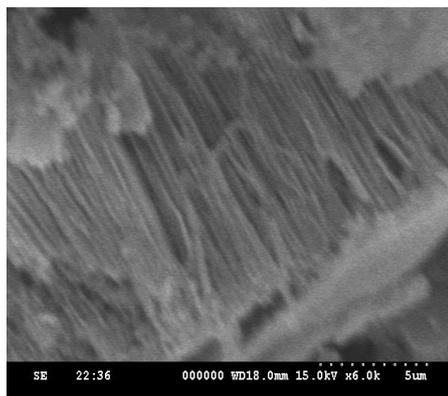
Figure 2. FESEM image of 1D LaFeO<sub>3</sub>-LaMnO<sub>3</sub> sample.
