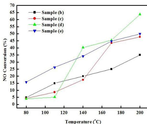
Figure 3. NO removal efficiencies of different LaFeO<sub>3</sub>-LaMnO<sub>3</sub> samples.
