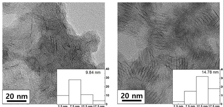
Figure 2. TEM images of MoS<sub>2</sub>(left) and WS<sub>2</sub>(right)
