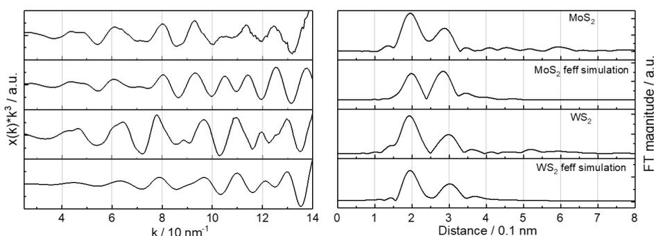
Figure 1. EXAFS spectra for the dispersed Mo and W catalysts
