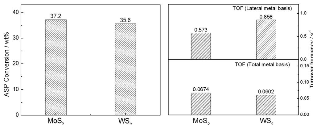
Figure 3. Comparison of asphaltene conversion and TOF over MoS<sub>2</sub>, and WS<sub>2</sub>
