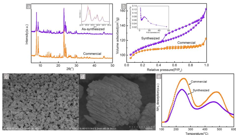
**Figure 1.** (a, b and c) XRD patterns,  $N_2$  adsorption-desorption isotherms, BJH pore diameter distribution curve (inset in b) and  $\text{NH}_3$ -TPD curves of the different ZSM-5 zeolites, (c and d) FESEM images of the synthesized ZSM-5 zeolite.
