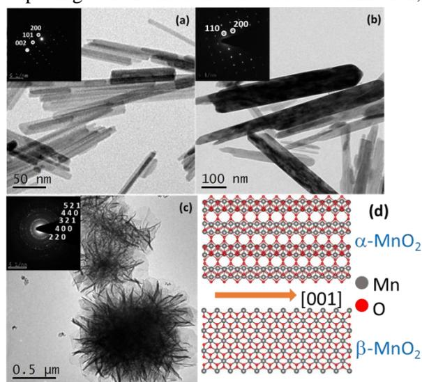
**Figure 1.** TEM bright field images of the catalysts: (a) α-MnO<sub>2</sub> nanorods, (b) β-MnO<sub>2</sub> nanorods and (c) α-MnO<sub>2</sub> flowers - their respective electron diffraction patterns are shown in the insets. (d) Schematic showing the atomic arrangements of [001]-oriented MnO<sub>2</sub> nanowires of the two different phases.
