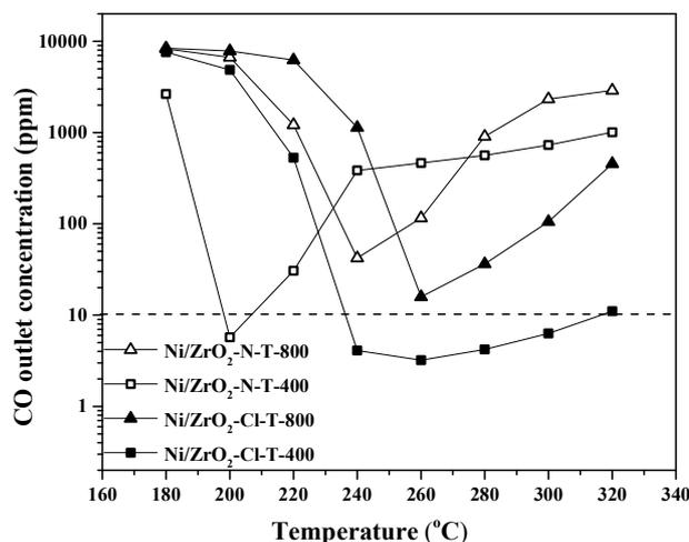
**Figure 1.** Catalytic activity for CO-SMET of the catalysts Ni/ZrO<sub>2</sub>.
