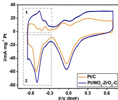
**Figure 4.** i-E profiles reduction of  $NO_3^-$  in Pt/C and Pt/ $WO_3$ - $ZrO_2$ -C. Supporting Electrolyte 1 M  $NaNO_3$  and 0.5 M NaOH. Scan Rate 20 mV/s.
