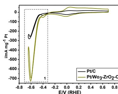
**Figure 5.** i-E profiles reduction of  $NO_2^-$  in Pt/C and Pt/ $WO_3$ - $ZrO_2$ -C. Supporting Electrolyte 1 M  $NaNO_2$  and 0.5 M NaOH. Scan Rate 20 mV/s.
