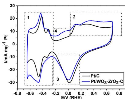
**Figure 3.** i-E profiles of the Pt/C and Pt/ $WO_3$ - $ZrO_2$ -C. Supporting Electrolyte NaOH 0.5 M. Scan Rate 20 mV/s.
