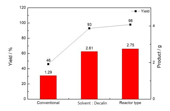
Fig.1. Product yield of  $\beta$ -naphthalene sulfonic acid
