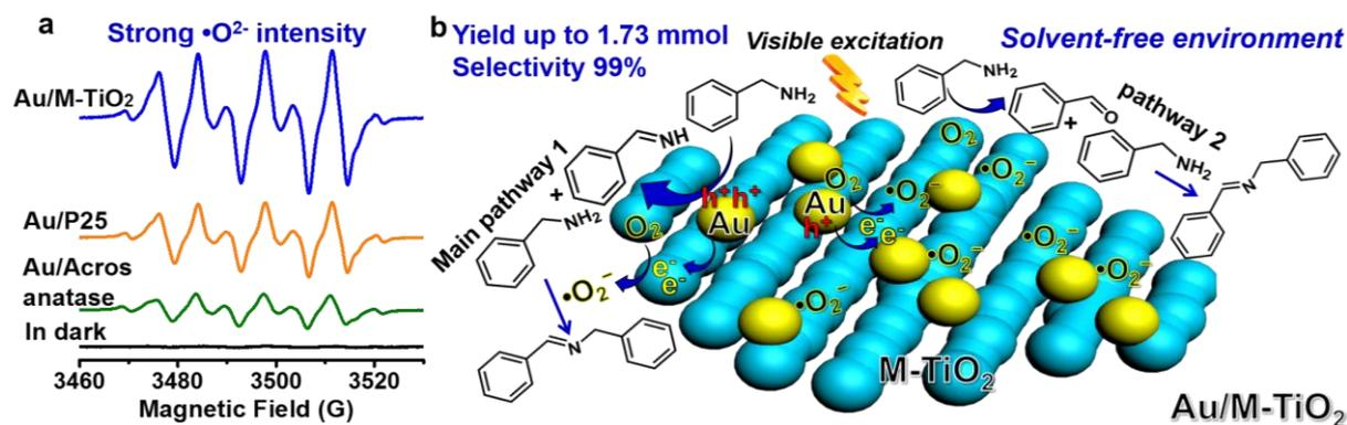
**Figure 2.** (a) DMPO spin-trapping ESR spectra of Au/M-TiO<sub>2</sub>, Au/P25 and Au/Acros anatase in methanol dispersion under visible light irradiation at ambient temperature and Au/M-TiO<sub>2</sub> in the absence of light, respectively. (b) Scheme of the proposed mechanism for selective aerobic oxidation of benzylamine to N-benzylidene benzylamine over Au/M-TiO<sub>2</sub> under visible light irradiation.
