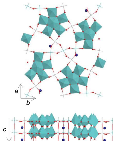
Figure 3. Structural model of MoVCuO. Ball in the structural model represents Cu.
